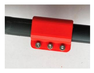
Next nip up the three screws to secure the two halves of the shaft. You do not need to over tighten.
