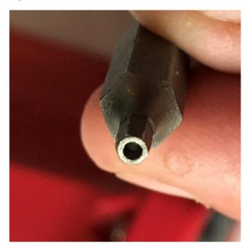
Once the screw is removed you can remove the shaft from the controller.
